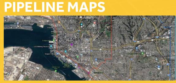
The red line in this image shows the location of a hazardous liquids pipeline in California and its proximity to specific roads, neighborhoods and critical facilities. Photo Credit: PHMSA
