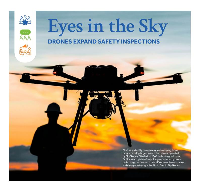
Pipeline and utility operators are testing drones fitted with cameras, lasers and sensors to enhance leak detection, inspect construction projects, patrol rights-of-way, identify geohazards and quickly respond following natural disasters such as wildfires, floods or tornadoes.
