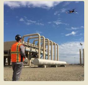
A Pacific Gas and Electric Company technician tests a methane gas sensor attached to a small drone. Photo Credit: Pacific Gas and Electric Company
